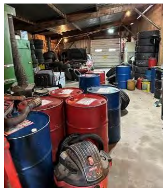
Photo No. 12 55-gallon drums of used oil for use in the used oil heater.
