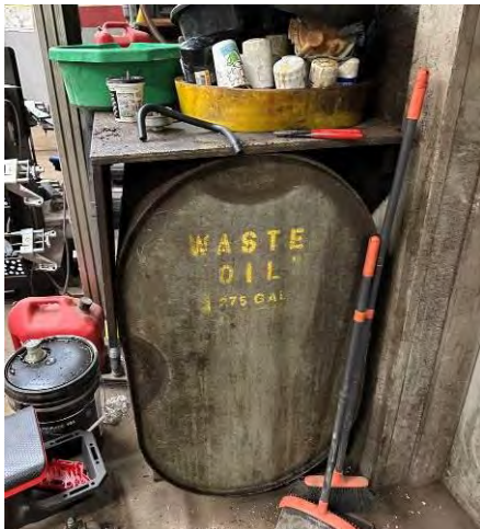
Photo No. 9 Waste oil AST stored along the southern wall of the garage bay.
