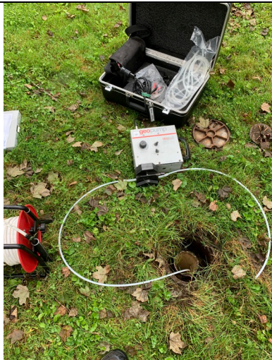
Photo 1: Photo of VFDC-MW-3S and set up during low-flow purging.
