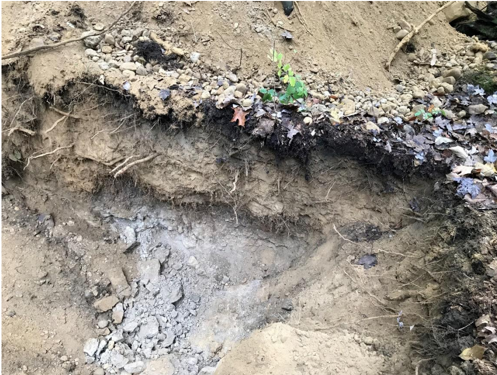
13.) Test Pit 10: Wall of test pit looking South. Bottom center of photo shows concrete block encountered.
