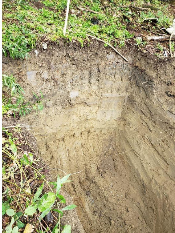
5.) Test Pit 3: Soil strata looking West.
